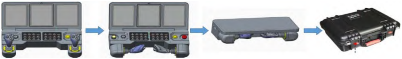
Figure 8. Structural design scheme of the main console of a remote control system for crane.
