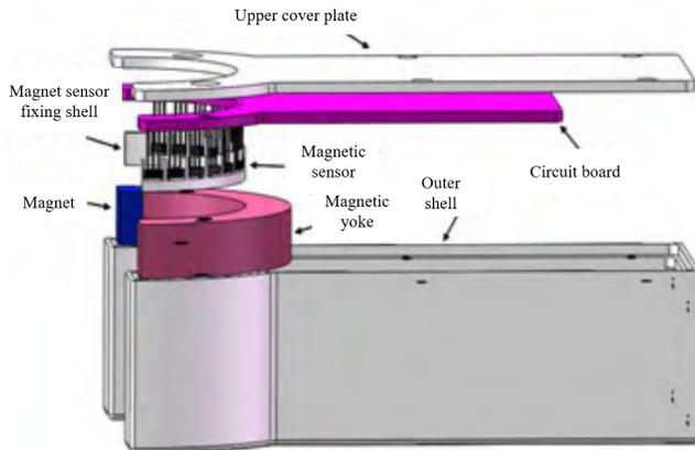
**Figure 3.** Three-dimensional diagram of the detection probe.
