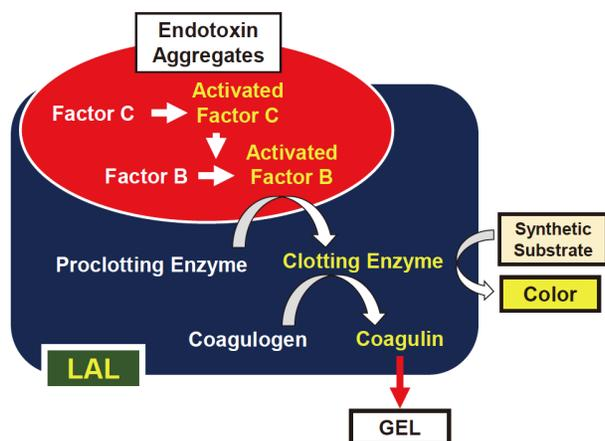
**Figure 1.** Cascade mechanism of the Limulus reagent<sup>[10]</sup>. Activation of Factor C and Factor B occurs on endotoxin aggregates and signal amplification takes place after activation of the proclotting enzyme.
