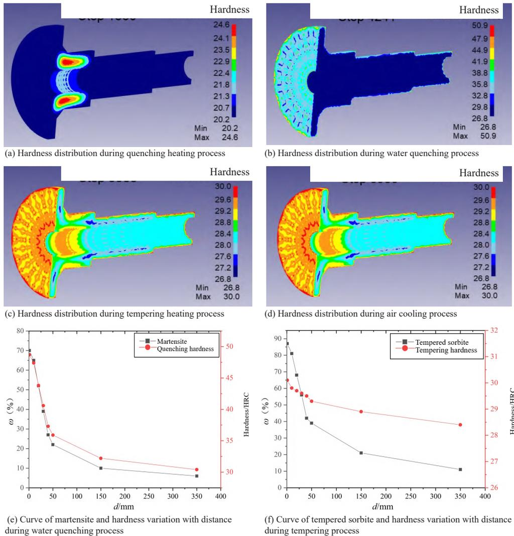
**Figure 6.** Changes in hardness field during heat treatment of the fan's main shaft
