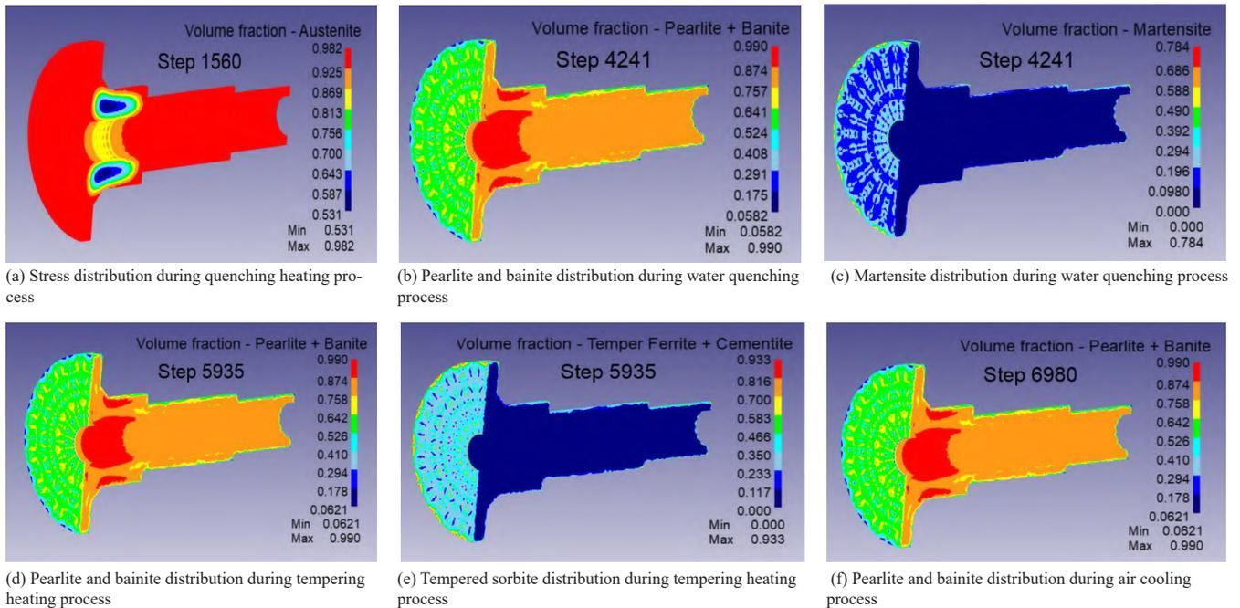
**Figure 5.** Phase field changes during heat treatment of the fan's main shaft
