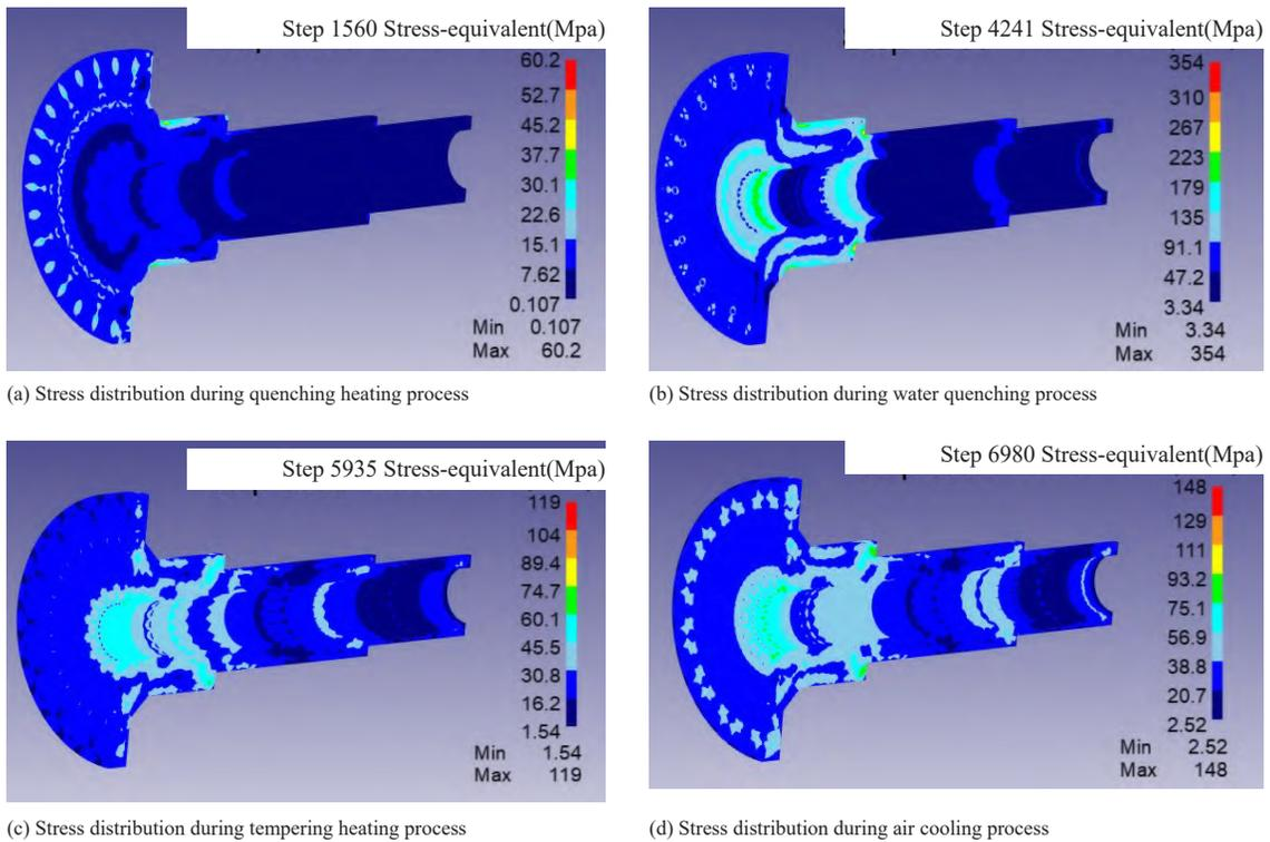
**Figure 4.** Changes in stress field during heat treatment of the fan's main shaft
