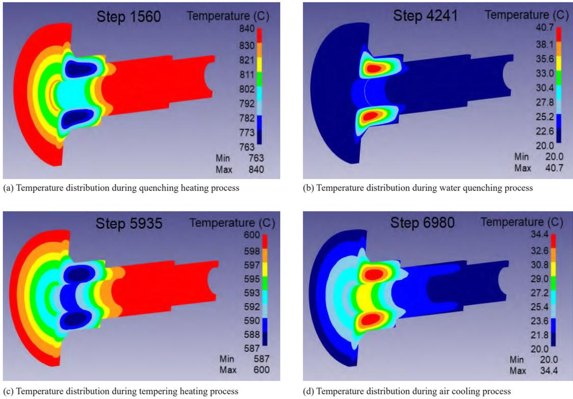
**Figure 3.** Temperature field changes during the heat treatment of the fan's main shaft
