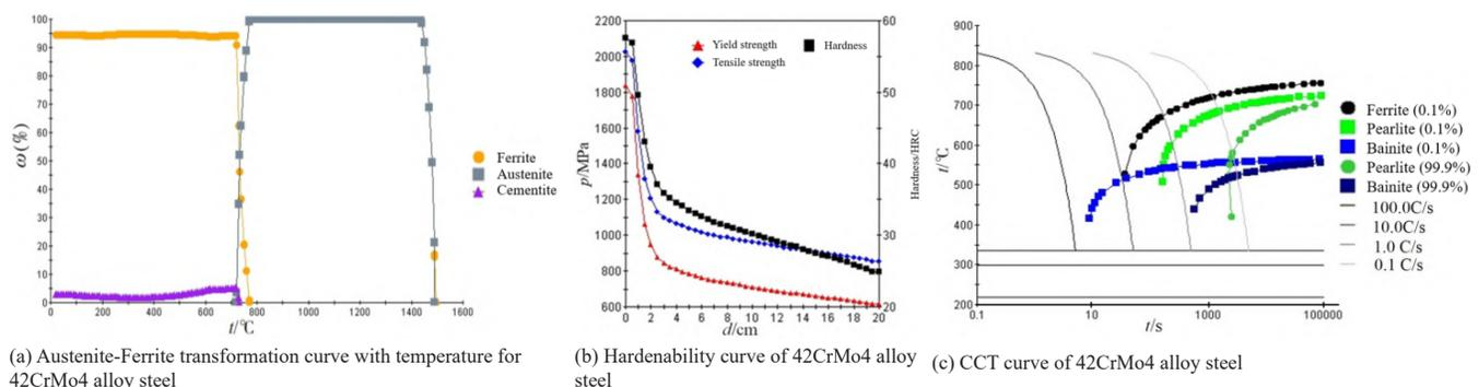
**Figure 1.** Basic data curves for heat treatment of 42CrMo4 material
