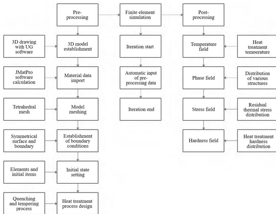
(a) Computer simulation of heat treatment process
