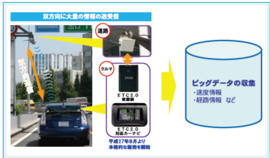
Figure 6. The collection of probe information through ETC2.0 onboard devices [8]
