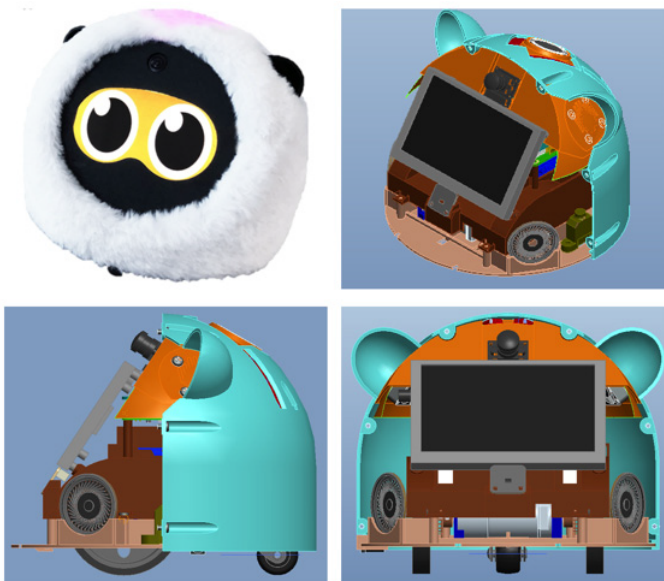
Figure 2. EDIE hardware CAD model and physical hardware
