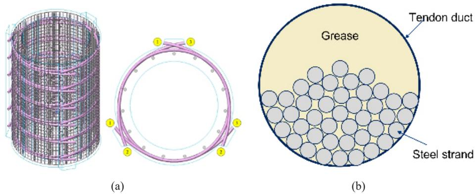
Figure 1. (a) Tendon duct locations in containment building; (b) cross-section of the tendon duct
