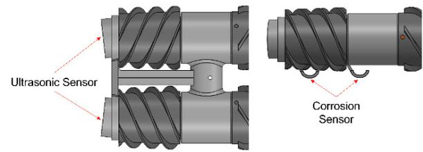
**Figure 3.** Modeling of the sensor mount
