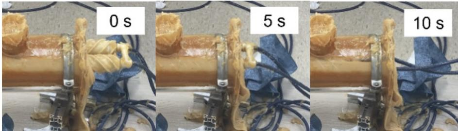
Figure 8. Robot propelling in grease
