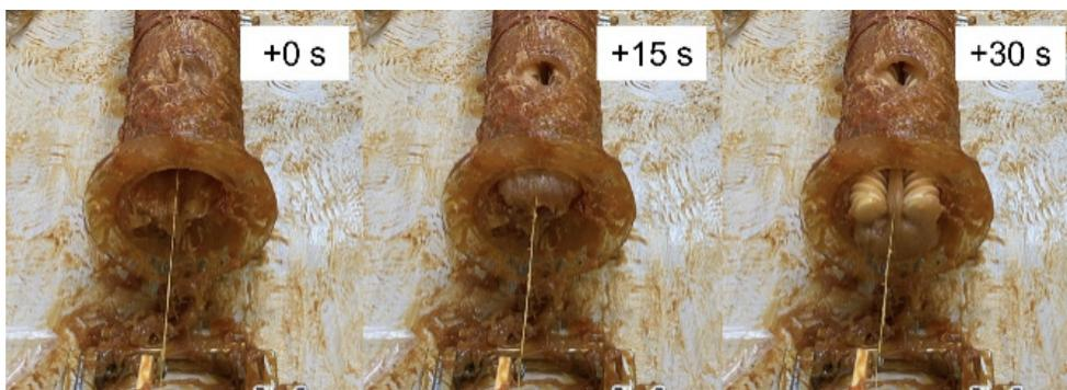
Figure 11. Robot passing through 6 m pipe, 15 sec interval
