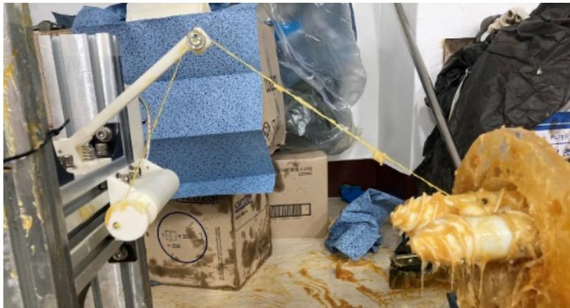
Figure 10. Winch to pull robot
