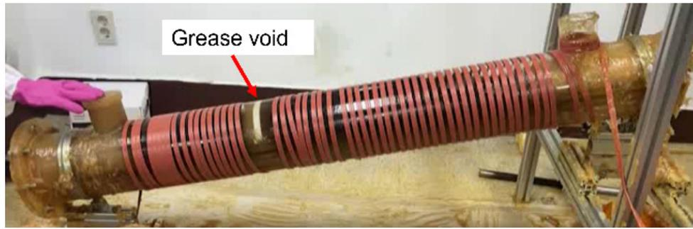
Figure 12. Sensor testing environment with grease void structure
