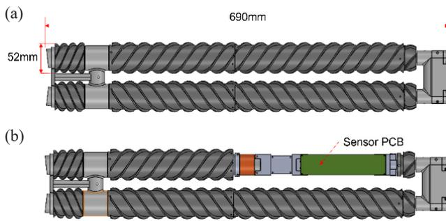
**Figure 2.** (a) Modeling of the screw-propelled robot; (b) printed circuit board (PCB) for sensor data communication
