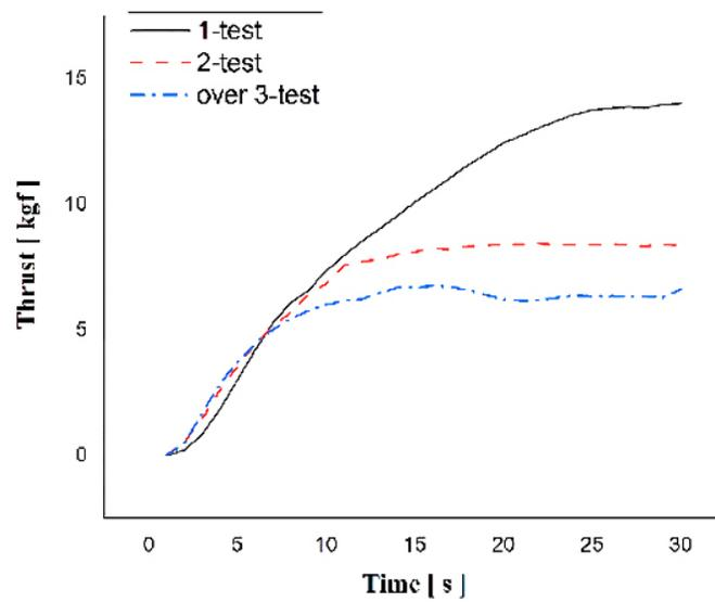
Figure 9. Propelling force of robot in grease
